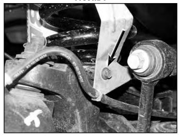
7. Remove the clips holding the front brake lines to the brackets on the frame. (Fig 2A) Using a proper line wrench, break loose the hard line at the junction block and rotate it 180 degrees. (Fig 2B) This will put the rubber line to the bottom. Tighten the hard line securely. Leave the brake line loose and save the retaining clip.
