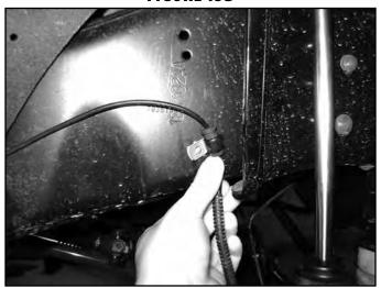
4" Lift Only: Remove the factory front brake line brackets from the frame. The brackets have a squared edge in the brake line mounting hole. (Fig 14A) Using a file or rotary grinder, remove the square edge to form a complete round hole. (Fig 14B) Reattach the brackets to the frame tighten securely with the factory hardware. Install the brake line junction in the bracket from the bottom and fasten with the factory retaining clip. (Fig 14C)
