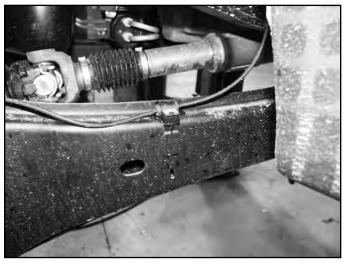
11. Disconnect the OE steering stabilizer from the frame mount.
