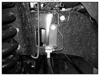
42. Properly bleed the brake system of air and top off the brake fluid reservoir with the proper type of fluid (see owners manual).
