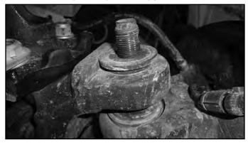
45. Remove the OE ball joint sleeve from the axle using the appropriate removal tool (SPC #41550 or equivalent) (Fig B).
