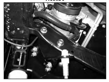
13. Position the stabilizer under the new bracket and install with the provided 12mm hardware (BP 657) and 3/4" steel spacer (YJTC5). (Fig 7) Torque to 50 ft-lbs.
