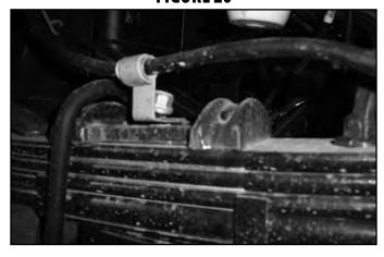
68. If more parking brake cable slack is needed, remove the cable from the rear-most retaining bracket on the frame. (Fig 21)
