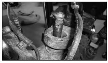
46. Install the new sleeve with the arrow on the top of the sleeve pointing toward the front of the vehicle. Using the old sleeve, pound down on the new sleeve to seat it on the ball joint taper. Make sure that the flat of the sleeve is flush with the flat of the axle (Fig C).
