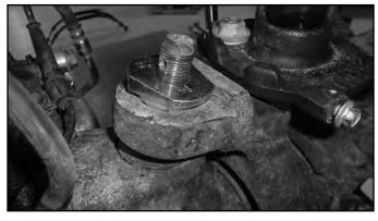
47. Install and torque the OE ball joint nut to 69 ft-lbs. Install the cotter pin. Note: Do not loosen the nut to install the cotter pin (Fig D).
