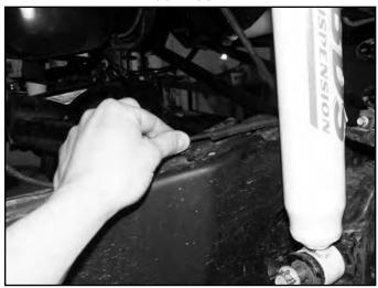
12. Install the new steering stabilizer bracket (01555) to the passenger's side of the engine crossmember using existing holes and new 1/2" x 1-1/4" bolts, nuts and washers (BP 657) (Fig 6). Mount the stabilizer bracket to the back side of the crossmember. Torque hardware to 55 ft-lbs.
