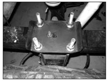
67. Repeat block installation of the driver's side. Take care not to over extend the brake lines.
