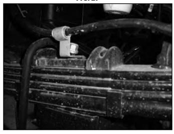
74. If more parking brake cable slack is needed, remove the cable from the rear-most retaining bracket on the frame. (Fig 28)
