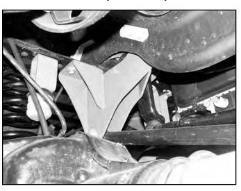
23. Pull the OE front bump stops free from the bump stop cups and remove the bolt mounting the cup to the frame (Fig 9).
