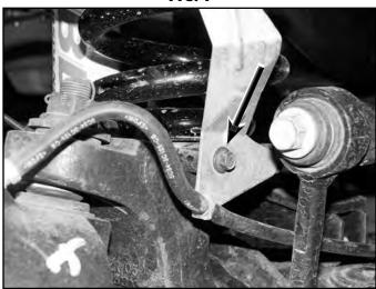
Remove the clips holding the front brake lines to the brackets on the frame. (Fig 2A) Using a proper line wrench, break loose the hard line at the junction block and rotate it 180 degrees. (Fig 2B) This will put the rubber line to the bottom. Tighten the hard line securely. Leave the brake line loose and save the retaining clip.
