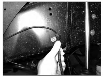
52. 4" Lift Only: Remove the factory front brake line brackets from the frame. The brackets have a squared edge in the brake line mounting hole. (Fig 21A) Using a file or rotary grinder, remove the square edge to form a complete round hole. (Fig 21B) Reattach the brackets to the frame tighten securely with the factory hardware. Install the brake line junction in the bracket from the bottom and fasten with the factory retaining clip. (Fig 21C)
