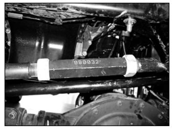
9. Disconnect the tie rod from the pitman arm, do not damage the tie rod boot. Mark the orientation of the pitman arm and remove the pitman arm from the sector shaft. (Fig. 3)
