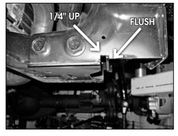
16. Place the radius arm drop bracket up to the frame rail. Insert ¾" bolt to locate the bracket. Mark the center of the slot on the bottom of the frame rail, mark the center of the top, rear hole on the side of the frame rail. (Fig. 8)
