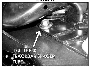
28. Fish the bolt tab through the frame rail with the included bolt wire and attach to the trackbar bracket with ½" USS washer and regular nut. Apply loctite to the bolt threads. Attach the upper hole with ½" x 1-3/4 (#792) bolt with spacer washer as shown. (Fig. 15A, 15B)
