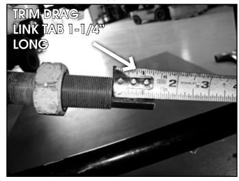
36. Reassemble the drag link, adjust so that there is approximately 3/4"~7/8" of thread exposed past the jam nuts and that the tie rod end faces up. (Fig. 18)
