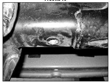
19. Place the machined sleeve into the existing frame rail hole. Reinstall the bracket with hardware (#793) and sleeve as shown. Torque 5/8" hardware to 150 ft lbs, 1/2" hardware to 80 ft lbs, and 3/4" hardware to 200 ft lbs. (Fig. 11A, 11B, 11C, 11D, 11E)
