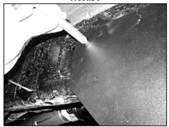
17. Remove the bracket and drill the 2 centers to 11/16". Prep the area on the side of the frame rail for welding. Place the weld in bung into the hole and weld the bung into place. (Fig. 9)
