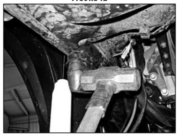
24. Grease new replacement bump stops and raise axle to press the bump stops into position. These will be a tight fit. It is easiest to lift the axle with a jack to compress the bump stops into position. (Fig. 13)
