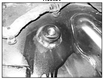
18. Insert the rivet nut into the bottom of the frame rail. Use the hardware (#799) to set the rivet nut into place as shown (Fig. 10) See the end of the instruction sheet for detailed rivet nut installation instructions.
