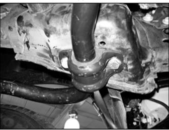
11. Disconnect the brake line bracket from the top of the radius arm mount on the axle, retain bolt, discard bracket. (Fig. 5)
