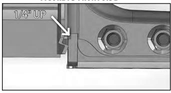
20. Remove the nuts from the transmission crossmember, if not already done in the transfer case index installation. Place the 4-link bracket up to the frame rail. Insert 3/4" bolt to locate the bracket. Mark the center of the slot on the bottom of the frame rail, mark the center of the top, rear hole on the side of the frame rail. (Fig. 8)
