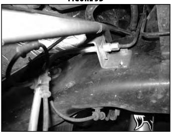
5. Disconnect the front driveshaft from the axle, retain the 4 bolts.
