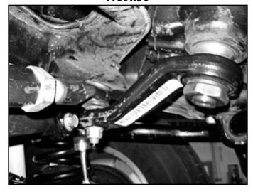
11. Disconnect the sway bar links from the sway bar they will not be reinstalled. (Fig. 4)
