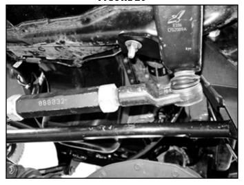
45. Route and attach the brakeline to the axle with factory hardware and clamps. (Fig 21)
