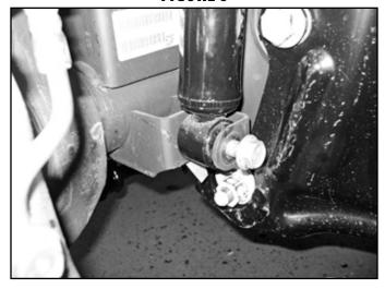
17. Raise the front axle and reattach factory shocks with factory bolt. It is not necessary to put the nut tab back on. The shocks will be there to keep the axle secure. Keep a jack under the axle for extra support.
