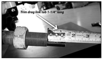
41. Reassemble the drag link, adjust so that there is approximately 3/4"~7/8" of thread exposed past the jam nuts and that the tie rod end faces up. (Fig. 18)
