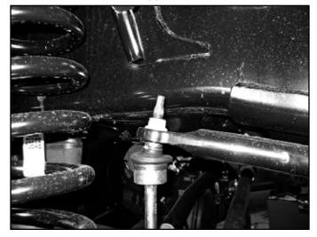
13. Disconnect the brake line bracket from the top of the radius arm mount on the axle, retain bolt, discard bracket. (Fig. 5)
