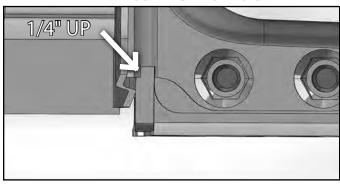
19. Remove the nuts from the transmission crossmember, if not already done in the transfer case index installation. Place the 4-link bracket up to the frame rail. Insert ¾" bolt to locate the bracket. Mark the center of the slot on the bottom of the frame rail, mark the center of the top, rear hole on the side of the frame rail. (Fig. 8)
