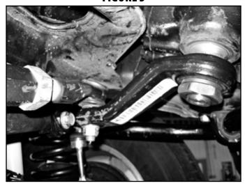
12. Disconnect the sway bar links from the sway bar. Retain all hardware. (Fig. 4)
