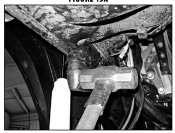
29. Grease new replacement bump stops and raise axle to press the bump stops into position. These will be a tight fit. It is easiest to lift the axle with a jack to compress the bump stops into position. (Fig. 13b)
