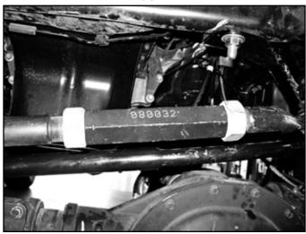
11. Disconnect the tie rod from the pitman arm, do not damage the tie rod boot. Mark the orientation of the pitman arm and remove the pitman arm from the sector shaft. (Fig. 3)
