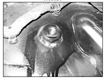
21. Insert the rivet nut into the bottom of the frame rail. Use the hardware (#799) to set the rivet nut into place as shown (Fig. 10). See the end of the instruction sheet for detailed rivet nut installation instructions.
