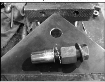
FIGURE 27- 1/2" RIVET NUT SHOWN
