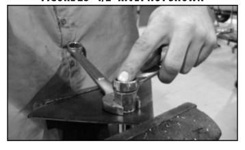
FIGURE 28 - 1/2" RIVET NUT SHOWN
