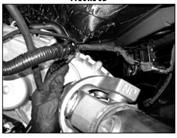
**Tip**Before hooking up the front driveshaft, now is a great time to grease the nearly impossible to access grease fitting on the front dual cardan joint. A needle adaptor on a grease gun is required. This fitting is required to be serviced at every oil change interval. Ensure that this maintenance is not skipped!
