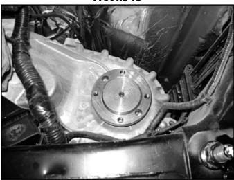
4. Disconnect the wire harness that controls the transfer case. (Fig 2a, 2b)
