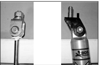
18. Grease bushings and sleeves and install into sway bar links. Install sway bar links with new 12mm hardware. (BP 795). Tighten to 45 ft-lbs. (Fig 11)
