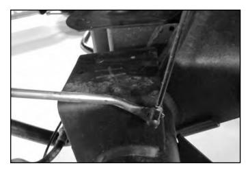
10. Disconnect the rear shocks and lower the axle, retain hardware. On the driver's side it is easiest to access the top hardware by cutting the inner fender well as shown. This trim procedure is not required but greatly aids in removal and installation of the shock (Fig 5a, 5b).
