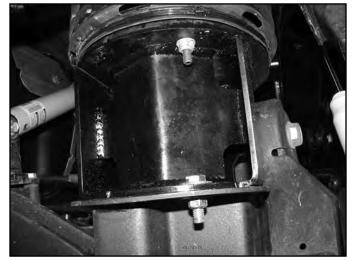
17. **3.5" - 5" Kit BDS NX2 Shock Installation:** BDS (Silver body) shocks will require a stem eliminator bracket to be installed and tightened on the shock before installation. The hardware is in bolt pack 946 included in the shock box. (Fig. 10 on Left)
