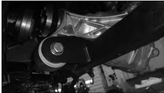
44. Reconnect the differential actuator wiring. Reattach the wire to the differential housing with the factory clips.
