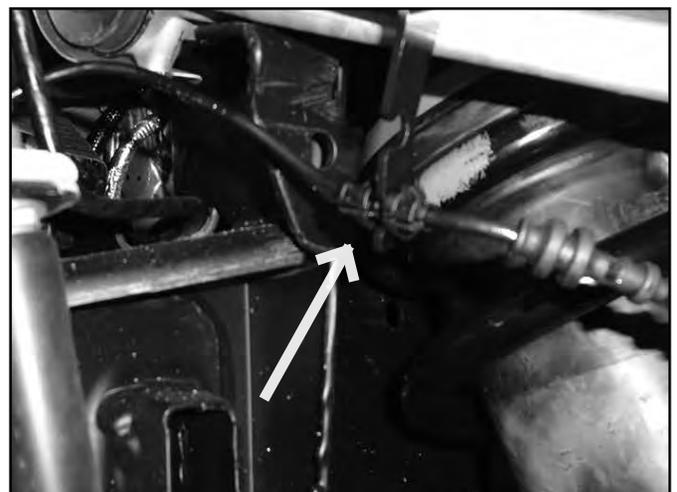
68. Attach the front sway bar to the sway bar drop bracket with the provided 3/8" bolts, prevailing torque nuts, and washers (Fig. 43). Attach the sway bar link to the front control arms. Torque the 3/8" bolts for the sway bar drop to 37 ft-lbs. Torque the sway bar link to the lower control arm to 74 ft-lbs.
