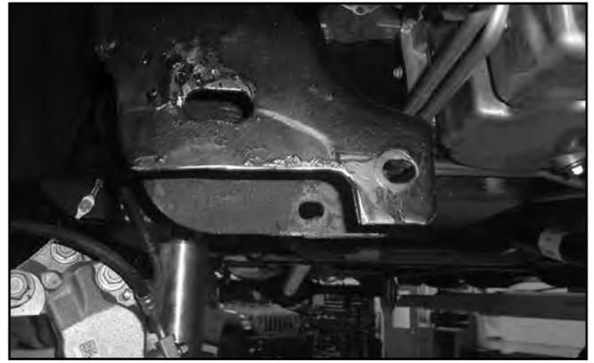
32. The bottom front of the front lower control arm pockets must be cut to provide clearance for the front cross member. This area needs to be cleaned of any oil, grease and/or undercoating. These coatings are flammable.
