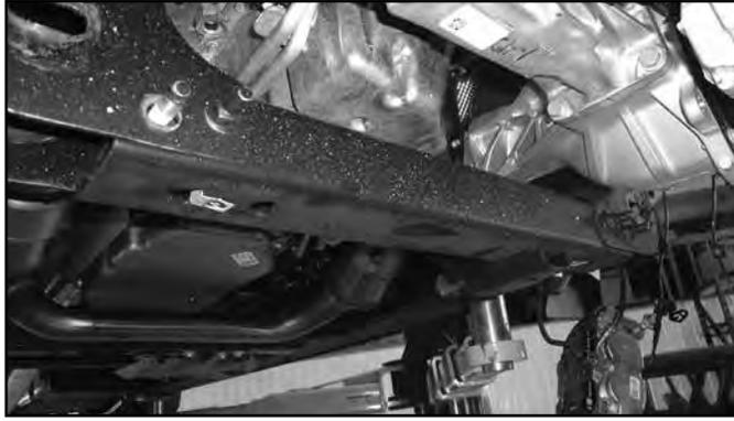
22. Disconnect the differential actuator wire connector from the actuator (Fig. 16).
