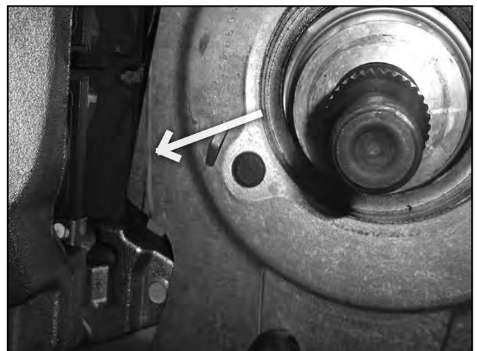
56. Install the modified dust shield on the corresponding new knuckles. Install the two O-rings on the new knuckle. Fasten the hub/shield with the OE bolts. Apply thread locker to the bolt threads and torque to 111 ft-lbs. with a final pass of 30-45 degrees per the factory specification.
