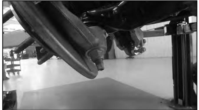
14. Mark each of the front strut bodies to indicate driver's versus passenger's side.
