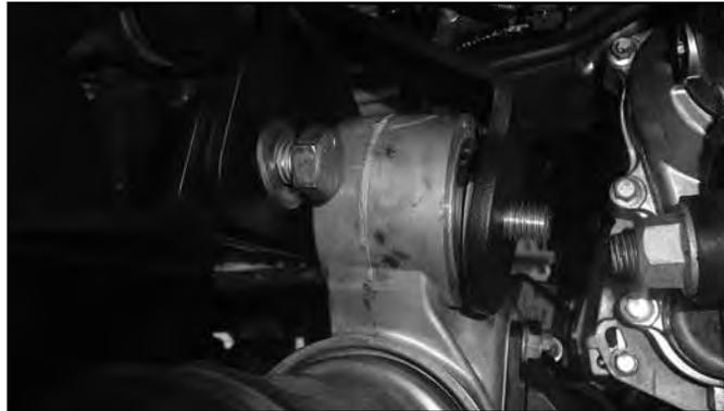
40. Install the provided sleeve through the slot on the factory rear cross member location. Attach the differential brace to the frame with the provided 1/2" x 5" bolt, prevailing torque nut, and washers (Fig. 28). Leave hardware loose.
