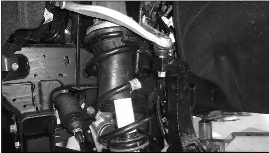
59. Torque the upper ball joint nut to 26 ft-lbs and then a final pass of 60-75 degrees per the factory specification. The lower ball joint nut should be torqued to 37 ft-lbs and then a final pass of 125-135 degrees per the factory specification.
