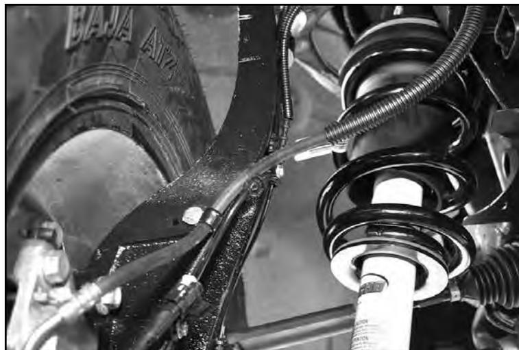
67. Attach the ABS wire and brake sensor wire to the upper control arm on the driver and passenger sides with the relocation bracket (03673 & 03674) and factory hardware using thread locker. The passenger side will use the lower hole of the relocation bracket (Fig. 42).
