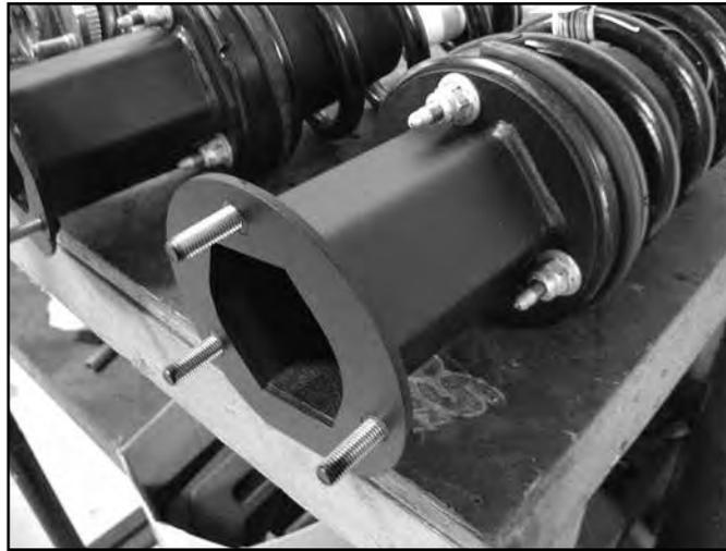
53. Install the new strut assembly to the appropriate frame mount with the factory nuts. Leave hardware loose.
