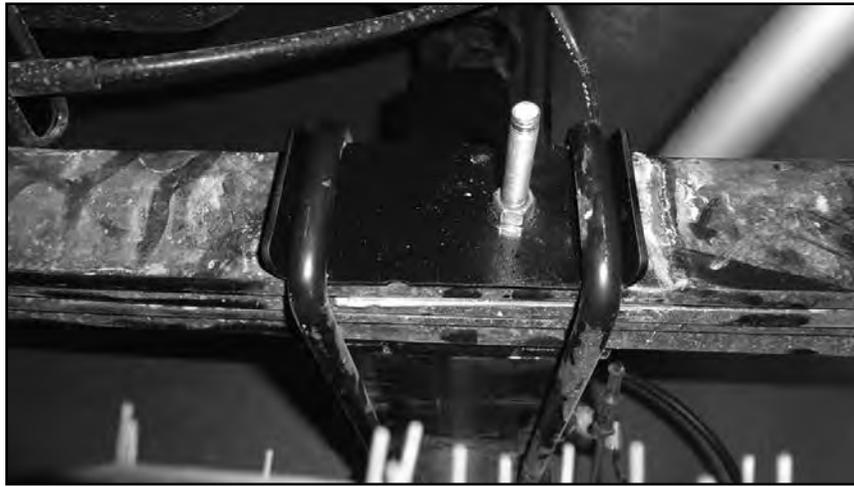
10. Start the nut on the center pin to hold the pack together but do not use the center pin to pull the leafs together. When the pack is completely together, torque the center pin to 30 ft-lbs. Remove the C-clamps.
