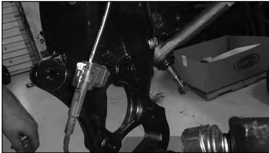
65. Attach the caliper to the new steering knuckle with the original mounting hardware and thread locker. Torque bolts to 37 ft-lbs with a final pass of 30-45 degrees per the factory specification.
