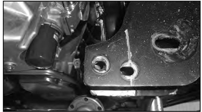
28. Make a vertical cut along each of the cut lines on the front and back faces of the control arm pocket with a reciprocating saw (recommended), cut-off wheel or plasma cutter. Be careful, the undercoating on the frame is flammable and can melt and drip off the frame. Keep a fire extinguisher near by.
