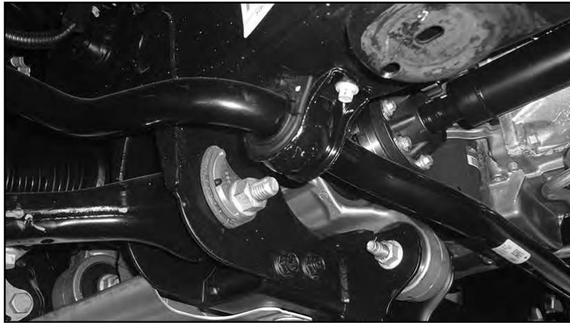
13. Remove the upper and lower ball joint nuts and thread back on by hand a couple of turns. **Aluminum Knuckles:** Avoid striking the knuckle to release the taper, a pickle fork or pry bar can be used to apply a splitting force. Gently hit the end of the ball joint to get it to release. If you do resort to hitting the knuckle avoid re-use and discard.
