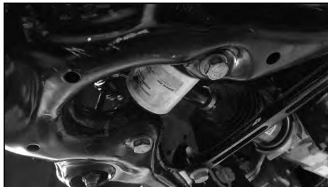
16. Remove the lower ball joint nut and remove the knuckle from the vehicle. Retain hardware.
