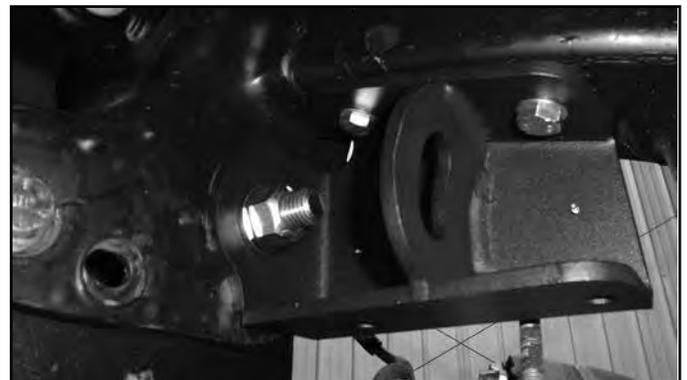
47. Install the OE lower control arms in the new cross members with the provided 18mm cam bolts, cam washers, and 18mm prevailing torque nuts. Run the front bolts from front to rear. Run the rear bolts from rear to front. Leave hardware loose. The main body of the cam will be 'up' in the cam slot.
