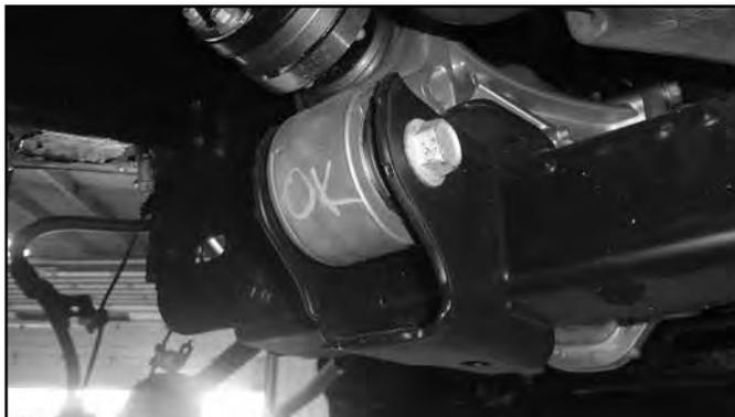
21. Remove the factory rear cross member from the vehicle by removing the 4 bolts. (Fig 15) Cross member and hardware will not be reused.
