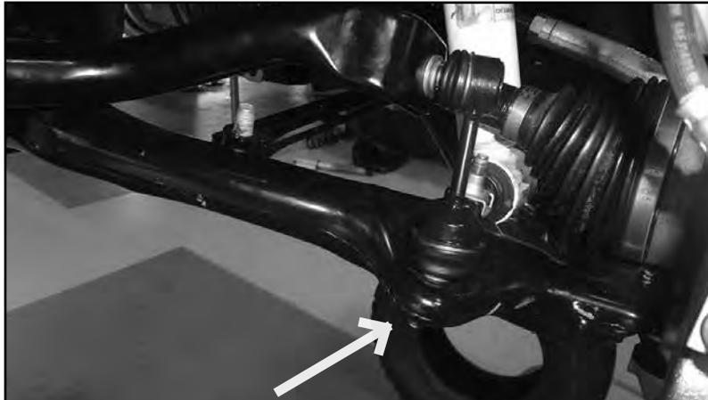
12. Mark the orientation of the sway bar and remove it from the frame by removing the four bushing cap mounting bolts (Fig. 8). Save all sway bar components, the hardware can be discarded..
