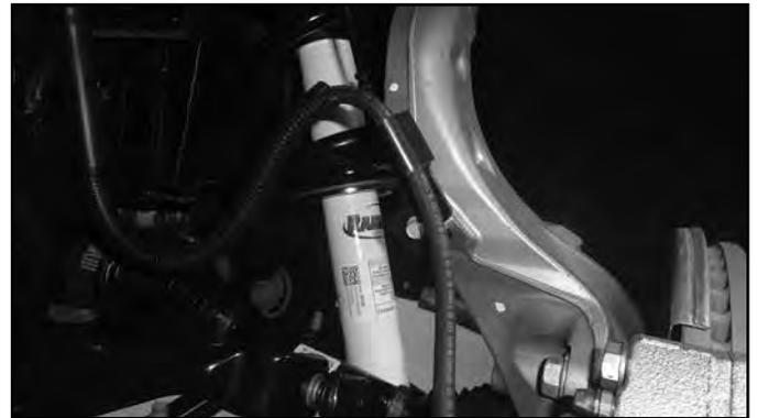
5. Remove the ABS sensor from the steering knuckle (Fig. 2).
