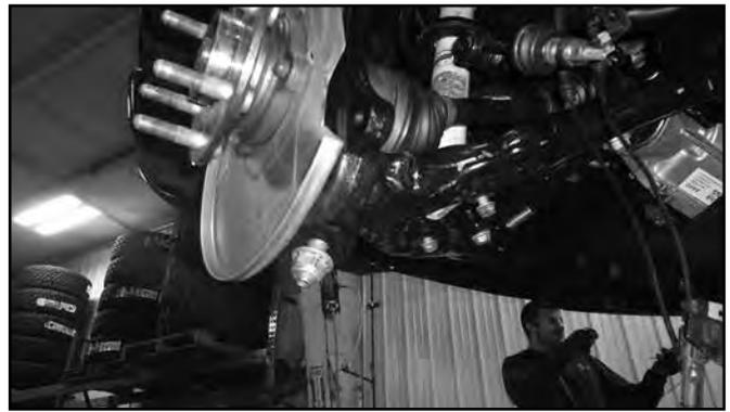
58. Attach the knuckle to the upper control arm with the original upper ball joint nut (Fig. 38).
