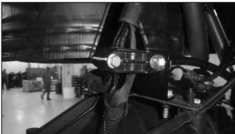
19. *4" Kit Only:* Reattach the brake and ABS brackets to the factory mounts and check for slack. The factory brackets may need to be bent to provide additional slack if needed.
