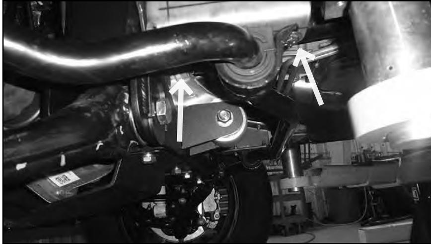
69. Connect the steering tie rod ends to the knuckles with the provided nylock nuts. Torque to 44 ft-lbs. Tighten the tie rod end jam nuts securely. They will be adjusted during alignment. Install the zerk fittings into the tie rod ends.
