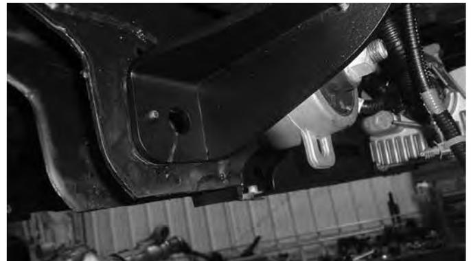
37. Install the front cross member (03615) in the control arm pockets with the the provided shorter 18mm bolt, prevailing torque nuts, and washers Run bolts from front to rear (Fig. 25). Leave hardware loose. Make sure to attach the differential bracket to the frame on the driver's side with the provided hardware.
