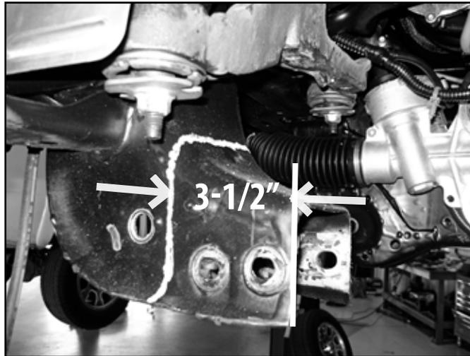
24. Make a vertical cut along each of the cut lines on the front and back faces of the control arm pocket with a reciprocating saw (recommended), cut-off wheel or plasma cutter. Be careful, the undercoating on the frame is flammable and can melt and drip off the frame. Keep a fire extinguisher near by.
