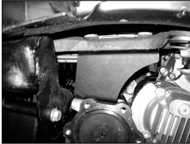
39. Install the differential to the new driver's and passenger's differential brackets. Fasten the differential to the driver side bracket with  $\frac{1}{2}$ " x 1-3/4" bolts, nuts and washers. Use the 5/8" bolt, 5/8" SAE washer and one extra thick 5/8" washer on the passenger's side. The extra large washer will go against the differential housing flange with the large slots. Leave hardware loose.
