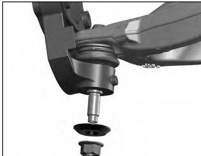
58. Attach the knuckle to the upper control arm with the original upper ball joint nut.
