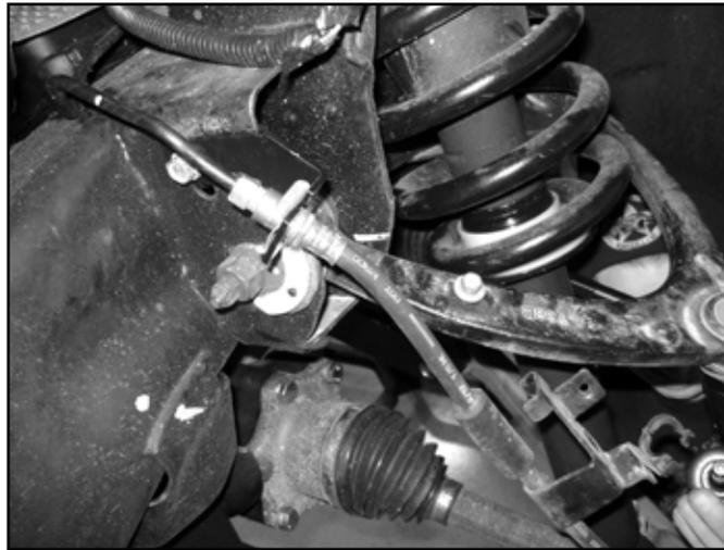
67. Carefully reform the brake hard line down so it meets the new bracket. Run the end of the rubber brake hose through the bracket and retain the brake line to the bracket with the original clip.
