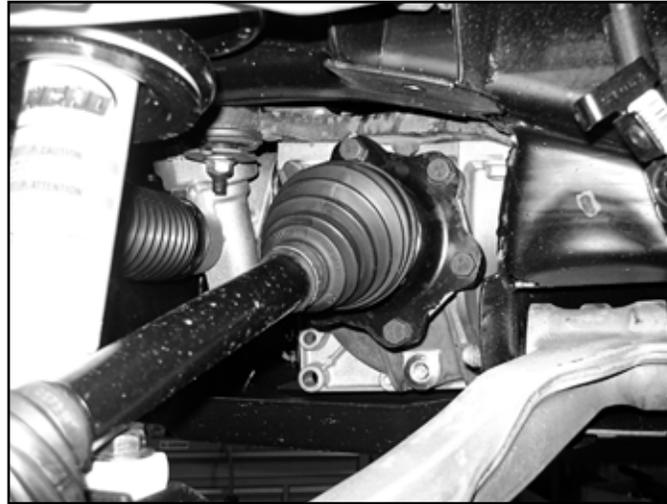
15. Remove the upper and lower ball joint nuts and thread back on by hand a couple of turns. **Steel Knuckle:** Strike the knuckle near the upper and lower ball joints to dislodge the tapered seat. **Aluminum Knuckle:** Avoid striking the knuckle to release the taper, a pickle fork or pry bar can be used to apply a splitting force. Gently hit the end of the ball joint to get it to release. If you do resort to hitting the knuckle avoid re-use and discard.
