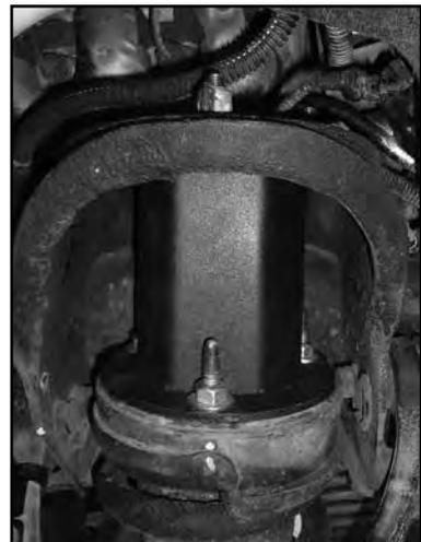
52. Install the strut assembly to the appropriate frame mount with the original nuts. Leave hardware loose. Make sure there is enough slack on the MagneRide wire harness.
