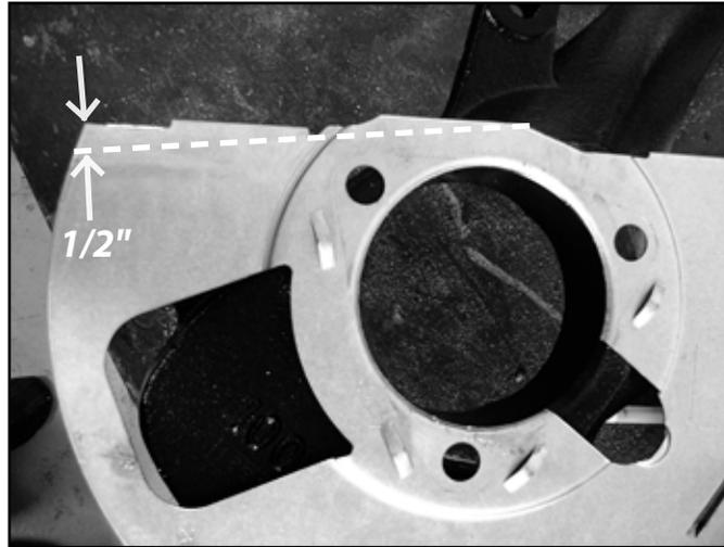
56. Install the modified dust shield and hub/rotor in the corresponding new knuckles. Fasten the hub/shield with the OE bolts. Apply Loctite to the bolt threads and torque to 133 ft-lbs. Be sure that the ABS line is run properly through the dust shield and out above the steering arm on the knuckle.
