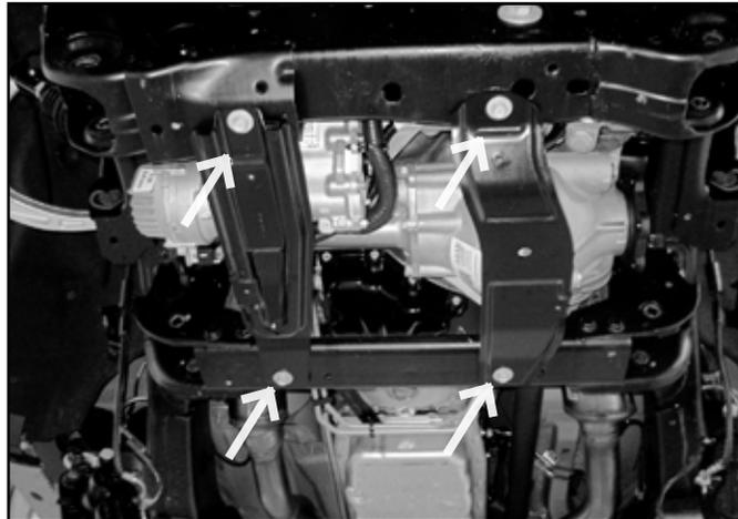
20. Remove the factory rear crossmember from the vehicle by removing the 4 bolts. (Fig 12) Crossmember and hardware will not be reused.
