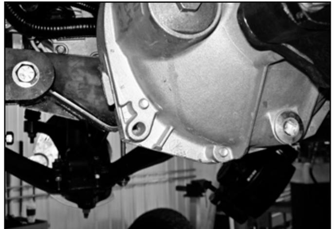
33. Locate the center differential bracket and 10mm x 40mm bolts and washers. Remove the 4 housing bolts and install the differential bracket with the provided hardware using some loctite. Torque bolts to 33 ft-lbs. Take care not to break the gasket seal. (Fig. 23)
