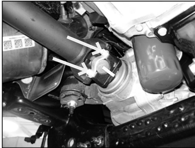
22. The driver's side rear lower control arm pocket must be cut to provide clearance for the front differential in the relocated position. This also aids in the removal of the differential. This area needs to be cleaned of any oil, grease and/or undercoating. These coatings are flammable.
