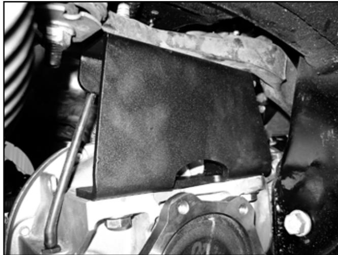
38. Install the new passenger's side differential bracket to the original mounting studs with the factory nuts (Fig. 28). The bracket is cleared for the electronic steering rack and mounts with the open face toward the inside of the vehicle. Torque nuts to 65 ft-lbs.
