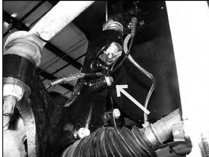
70. Attach the front sway bar to the original mounts in the stock orientation in conjunction with the provided drop brackets (02166B - 6.5" kit, 02491 - 4.5" kit) and 10mm bolts/washers (10mm x 120mm - 6.5" kit, 10mm x 80mm - 4.5" kit). Use Loctite on the bolt threads and torque to 45 ft-lbs. (Fig. 37)
