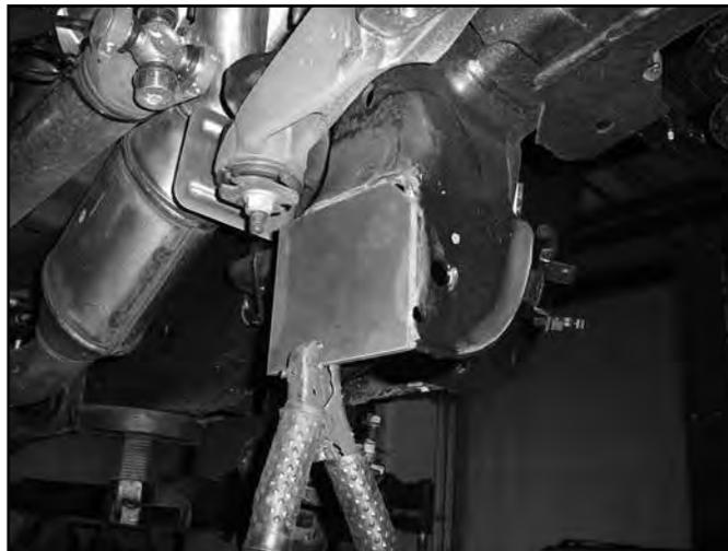
35. With the plate tacked, go back and weld the plate in place. Weld along the OUTSIDE of the pocket on the vertical surfaces. Welding on the inside will result in crossmember interference. Weld along the top edge of the plate on the inside of the pocket. Once the area has cooled, paint all exposed metal to prevent corrosion.
