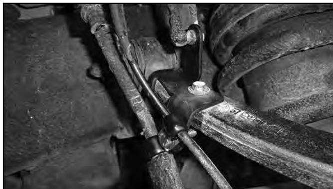
69. Reconnect ABS line at the frame. Attach the ABS line to the steering knuckle with the provided wire clamps and  $\frac{1}{4}$ " x  $\frac{3}{4}$ " self tapping bolt and flat washer. Torque bolt to 15 ft-lbs. Use zip ties to retain the remaining section of the ABS line as needed to keep it away from rotating objects. (Fig. 36)
