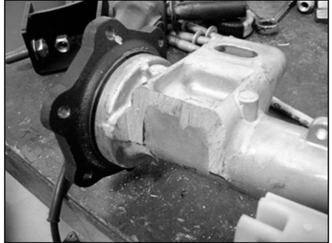
30. Clean up the cuts with a sanding disc or flap wheel. Be sure to remove the remaining material on the outside flange so it matches the rest of the contour. (Fig. 20)
