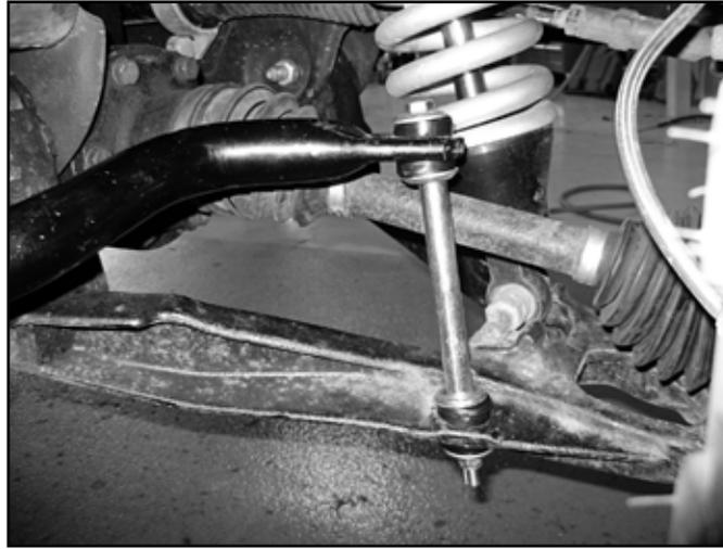
72. Connect the steering tie rod ends to the knuckles with the short provided nylock nuts. Ensure the nut has full thread engagement. Torque to 60 ft-lbs. Tighten the tie rod end jam nuts securely. They will be adjusted during alignment. Install the zerk fittings into the tie rod ends.
