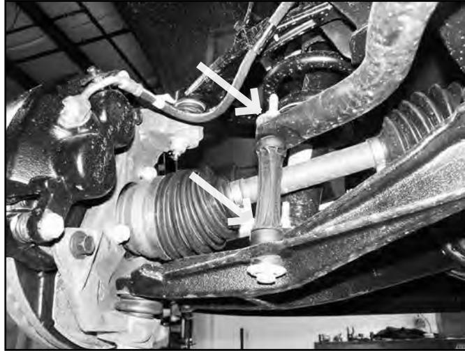
11. Mark the orientation of the sway bar and remove it from the frame by removing the four bushing cap mounting bolts (Fig. 7). Save all sway bar components.
