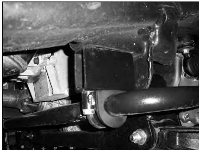
71. The new sway bar links will be built from a 5" sleeve,  $\frac{3}{8}$ " x 9" bolt, bushings and cup washers. Attach these to the sway bar followed by the control arm with the bolt going from the top down. (Fig. 38) Tighten the sway bar link until the bushings begin to form to the control arm surface.
