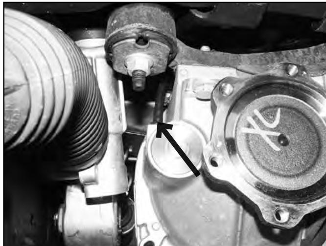
28. Support the front differential with an appropriate jack. Remove the two driver's side differential mounting bolts (Fig. 17) and the two passenger's side mounting nuts. Carefully lower the differential to the ground. Save mounting hardware.
