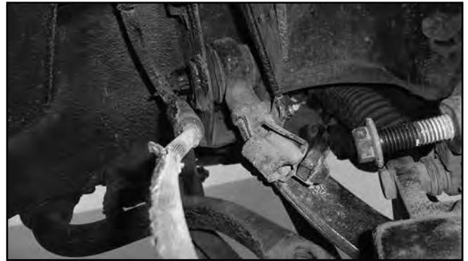
5. Remove the splash guard from the vehicle. (Fig 2)
