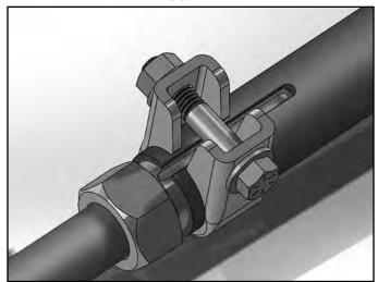
35. Using a 5/8" socket and 11/16" wrench, tighten the pinch bolt to 40 ft-lbs.
