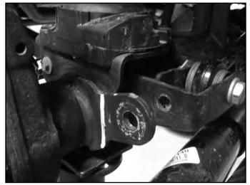
22. Attach the short mounting post into the original sway bar link mount hole on the track bar bracket. Tighten the post ensuring the click pin hole is horizontal or parallel with the ground. Tighten to 65 ft-lbs. (Fig 8)
