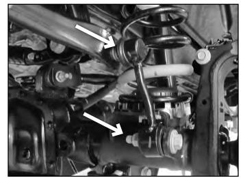
8. Disconnect the brake lines from the control arms to allow enough slack for coil removal (Fig 4). Support the front axle with a hydraulic jack. Remove the front shocks from the vehicle. Retain upper and lower mounting hardware.
