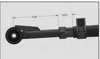
34. Ensure that the clamp is located 1/2" from the end of the tube, facing up. This is to avoid contact with other suspension/ steering components. Also ensure that the clamp is centered upon the slit on the end of the tube. Both the slit on the tube and the slit on the hex adjustment collar must be perfectly aligned. This is illustrated in Figure 14 below.
