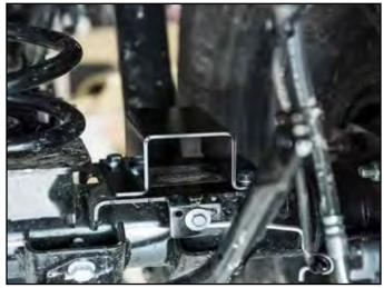
45. Install the hourglass bushings and sleeves into the shocks. Fox shocks install with the body up, NX<sup>2</sup> shocks install with the body down. Install using the factory hardware, torque the upper and lower bolts to 89 ft-lbs
