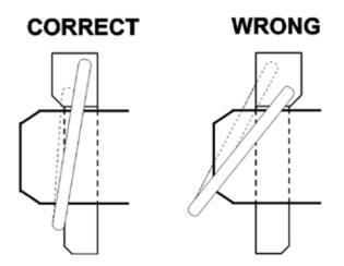
When properly installed, the ring on the Click Pin will "snap" against the shaft of pin. When installed backwards, the ring does not fit snugly against shaft.
