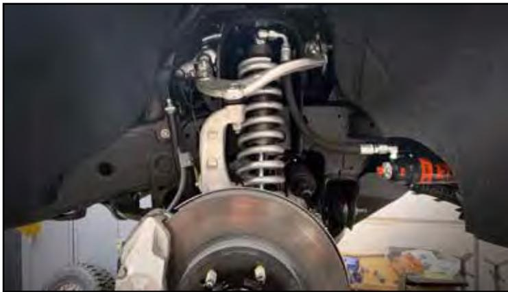
29. Reattach the brake wire / ABS wires to the factory position on the knuckle. Use the provided wire clamps and 1/4" bolt to attach the brake wire / ABS wire to the upper control arm. Check for enough slack in the wires and adjust as necessary.
