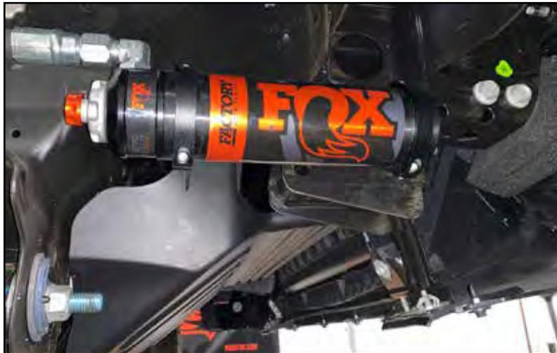
23. Install the remote reservoir bracket using the factory skid plate bolt. Ensure that the remote reservoir bracket is installed under the skid plate. The larger hole on the bracket goes toward the rear of the vehicle. Torque the splash shield bolt to 16 ft-lbs. (Fig. 15).
