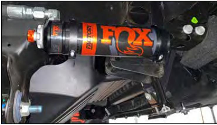
28. Installed coil-over will resemble Figure 18. (BDS UCA not shown)
