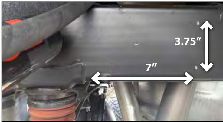
24. Install the bracket using one of the  $\frac{1}{4}$ " self-tapping screws to partially install the reservoir bracket. Ensure that you mount the bracket so that the forward most hole is the side that has the screw installed (Fig. 31).
