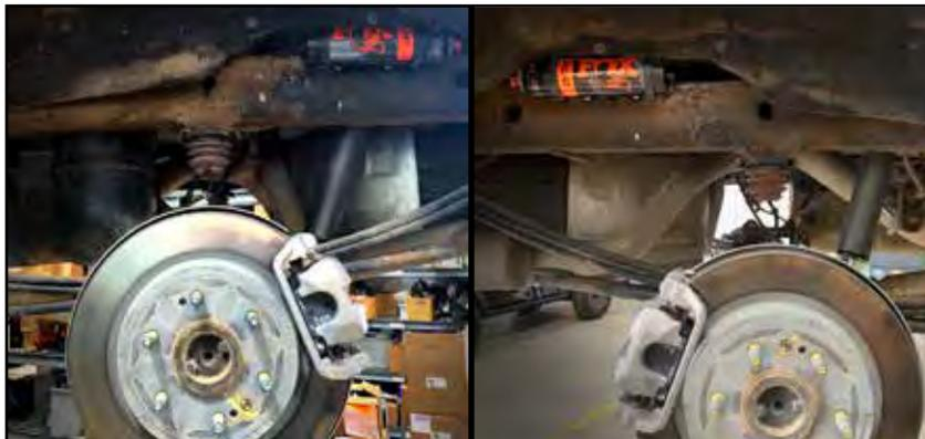
23. To install the rear reservoir brackets, you must drill a 7/32" hole that is 7" away from the edge of the OEM bump stop mount toward the rear of the vehicle and 3-3/4" above the bottom of the frame rail (Fig. 30).
