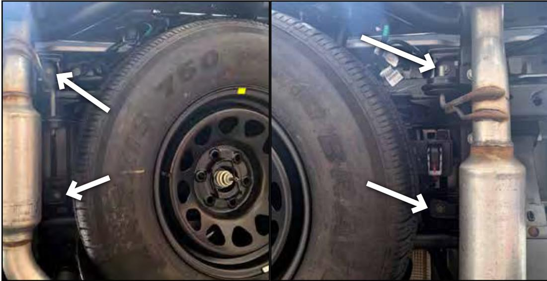
15. Loosen the (2) most forward bolts of the bed. DO NOT remove. These bolts keep the bed aligned while you lift the rear of the bed to slide the reservoirs between the bed and the frame rail (Fig. 22).
