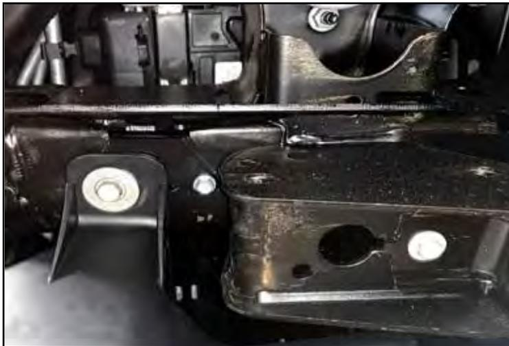
25. Now fully install the reservoir bracket onto the vehicle using the supplied 3/4" self-tapping screws.
