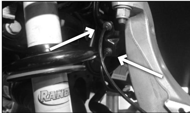
8. Support the lower control arm with a hydraulic jack. Remove the upper ball joint nut and thread back on a couple of turns by hand. Separate the upper ball joint from the steering knuckle, use of a ball joint separation tool to dislodge it from the knuckle is recommended. (Fig. 5A) Remove the nut and remove the ball joint from the knuckle. Allow the knuckle to rest back away from the front strut.
