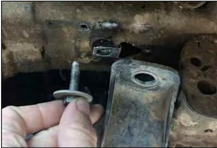
24. Using a 7/32" bit, drill a pilot hole for the provided self-tapping screw. This screw goes through the smaller hole on the reservoir bracket. This screw prevents rotation of the reservoir bracket (Fig. 16).
