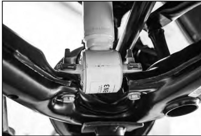
10. Remove the three nuts attaching the strut to the frame (Fig. 7). Remove the strut from the vehicle. DO NOT remove the center strut rod nut. Discard the nuts, they will not be reused.
