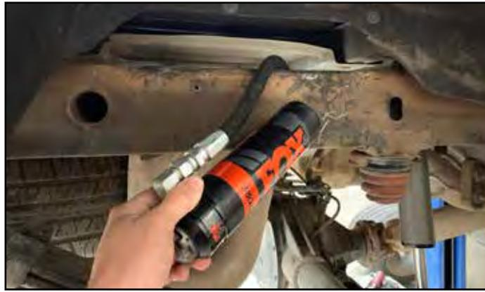
19. Once the reservoirs have been slid between the frame and the bed of the vehicle, slowly lower and reattach the bed to the vehicle using the OEM hardware. Torque the box hardware to 63 ft-lbs.
