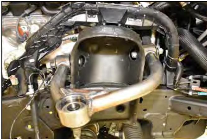
14. Attach the ball joint on the new upper control arm to the knuckle. Snug up hardware, but do not tighten down.
