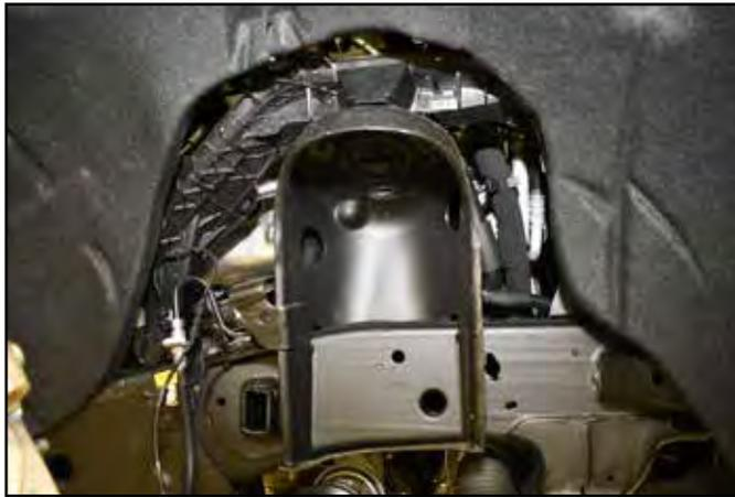
12. Cut the factory droop limiter from the side of the strut bucket as shown in Figure 9.
