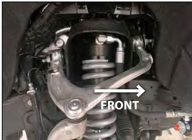
18. Connect the coil-over to the lower control arm using the supplied 10mm bolts and washers. Torque to 50 ft-lbs.
