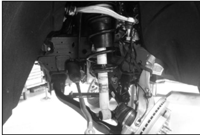
9. Remove the two lower strut bar pin bolts (Fig. 6). The bolts will not be reused. Lower the control arm with the jack so there is enough room to remove the factory strut.
