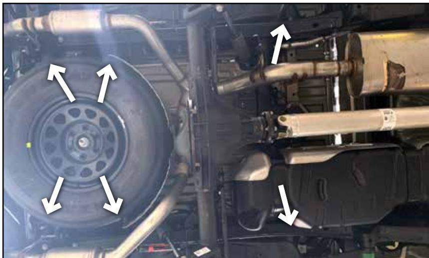
14. Remove the rear bolts attaching the bed of the truck to the frame. DO NOT discard bolt bolts, as they will be used to reinstall the bed (Fig. 21).
