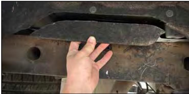
22. The remote reservoirs mount to the vehicle using supplied mounting brackets toward the back of the vehicle in the wheel arch (Fig. 29). The left image in Figure 29 is the driver side and right image is the passenger side.
