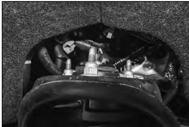
11. Remove the ABS wire / brake sensor wire from the upper control arm. Remove the upper control arm from the vehicle by removing the two bolts attaching the upper control arm to the strut bucket / frame (Fig. 8). Save hardware. If replacing the upper arm on a Denali truck, remove the sensor arm from the ball stud on the upper control arm.
