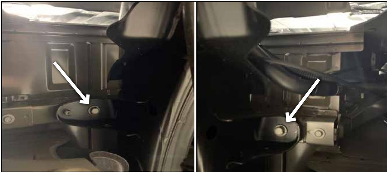
16. Once bed bolt removal is complete, slowly lift the rear of the bed from underneath the bed plate (Fig. 23). Lift the bed  $\frac{3}{4}$ " from the frame rail (Fig. 24). DO NOT lift the bed from underneath the bedside as this may cause damage to the bedside. Be sure to check that the bed does not contact the cab of the truck as this could cause damage to the bed and the cab of the vehicle (Fig. 25).
