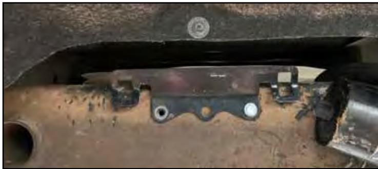
25. Using the bracket as a guide, drill a  $\frac{7}{32}$ " hole through the rear most hole of the reservoir bracket. Install the remaining  $\frac{1}{4}$ " self-tapping screw to fully install the reservoir bracket. There should be (2) two self-tapping screws in each bracket (Fig. 32).
