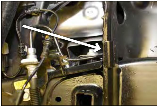
13. Install the new upper control arm to the vehicle using the factory hardware with the bolts running from the inside out (Fig. 10) Snug up hardware.
