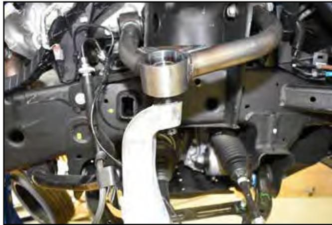
20. Reattach the tie rod to the knuckle and torque the factory nut to 44 ft-lbs.
