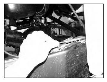
11. Remove the two bolts mounting the plastic ABS wire clips to the back side of the coil perch (Fig 5). Retain hardware.
