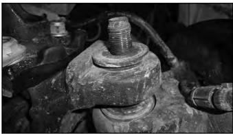
18. Remove the OE ball joint sleeve from the axle using the appropriate removal tool (SPC #41550 or equivalent) (Fig B).
