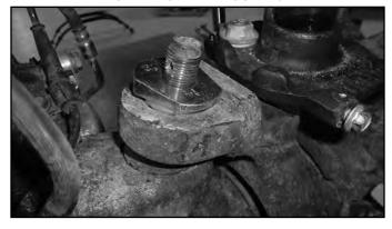
20. Install and torque the OE ball joint nut to 69 ft-lbs. Install the cotter pin. Note: Do not loosen the nut to install the cotter pin (Fig D).
