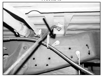
49. The brakelines may require additional slack. Located the factory bracket on the axle. Using an adjustable wrench, carefully bend the bracket so the fittings are positioned vertical to allow more slack. (Fig 14)
