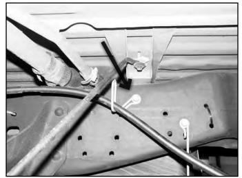
43. The brakelines may require additional slack. Located the factory bracket on the axle. Using an adjustable wrench, carefully bend the bracket so the fittings are positioned vertical to allow more slack. (Fig 14)
