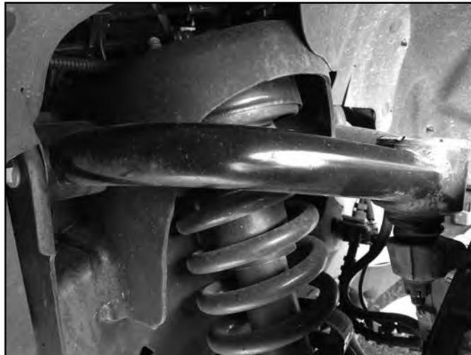
9. Grease the ball joint at this time.
