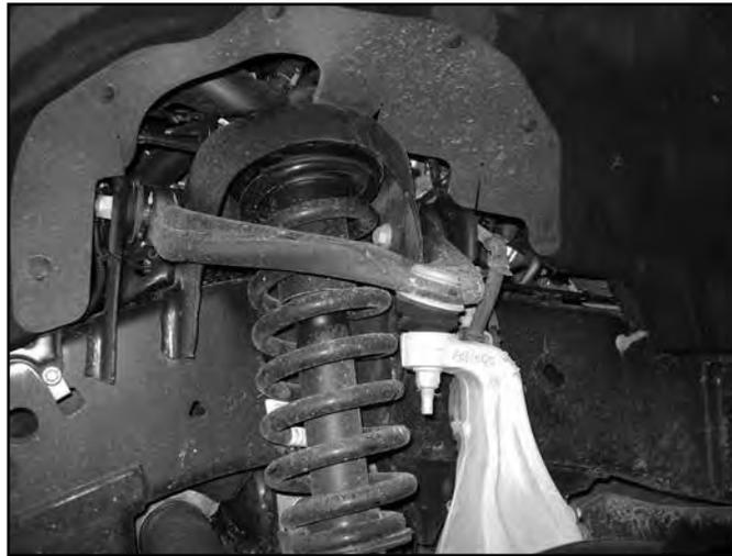
5. Remove the upper control arm from the vehicle and retain the upper control arm hardware.
