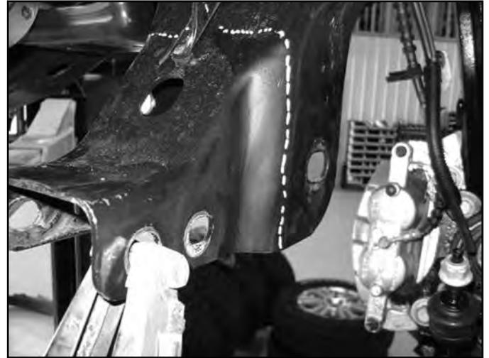
26. On the back side measure from the inside edge of the slot 1-3/4" and make and mark a vertical cut. Measure 1" in from the angled top surface and mark (Fig 15).
