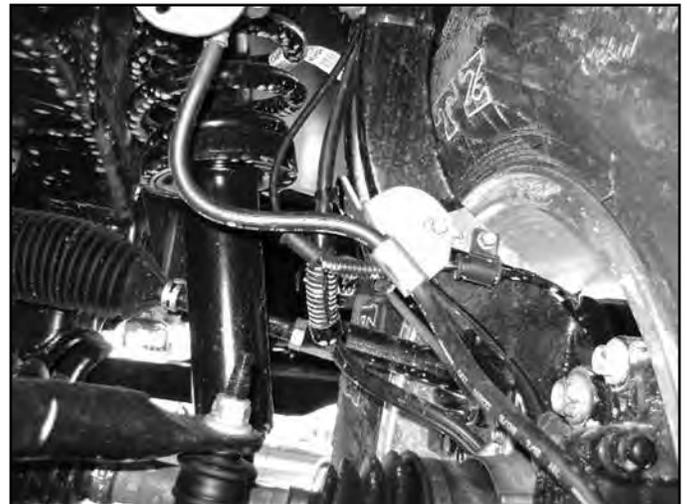
58. Install the sway bar to the new sway bar drop brackets with 7/16" x 1-1/4" bolts, nuts and 7/16" SAE washers (BP #772). Attach the sway bar to the sway bar end links with the original hardware. Torque the 7/16" hardware to 45 ft-lbs. Torque sway bar link nut to 45 ft-lbs.
