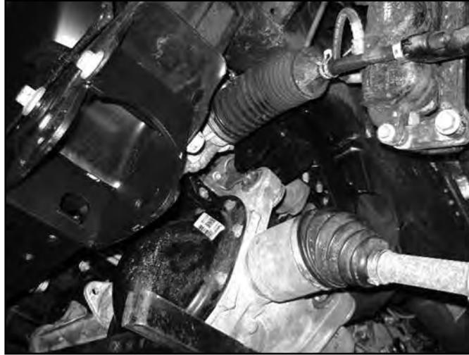
29. Install the new rear cross member (02780) in the rear lower control arm frame pockets. Attach the rear cross member with the sway bar drop brackets (02781) with new 18mm bolts and washers (BP #773). Run bolts from rear to front (Fig 22A). Leave hardware loose. Ensure the cutout made in Figure 15 is adequate to clear the differential mounting bolt. (Fig 19A). Do not tighten hardware at this time.
