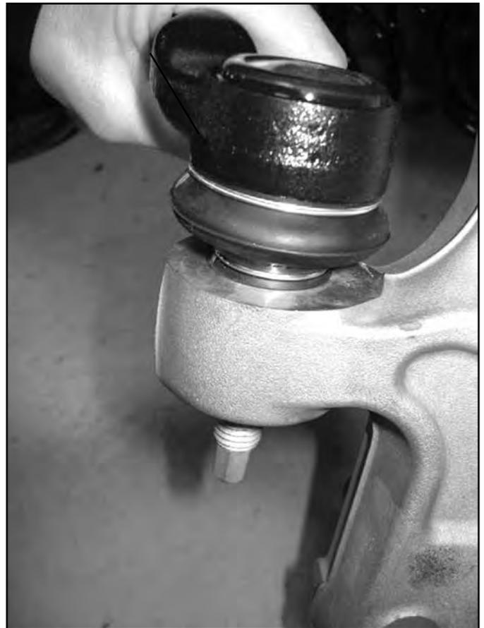
11. Disconnect the sway bar links from the sway bar (Fig 5). Retain hardware. The sway bar links do not need to be removed from the lower control arms.
