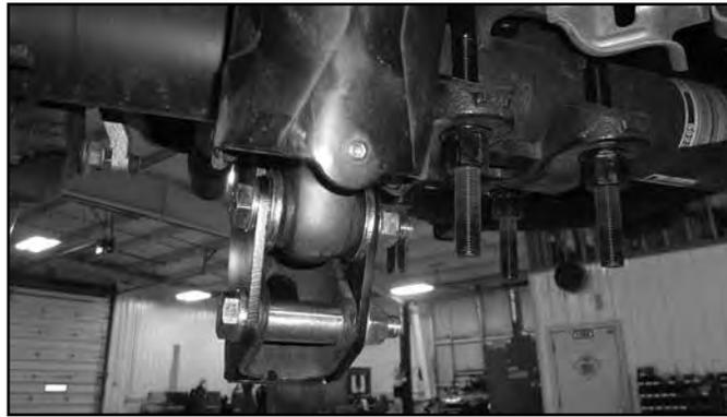
81. Install the provided brake line relocation bracket to the driver's side frame rail with the OE brake line bracket bolt (Fig 37). Torque to 15 ft-lbs.
