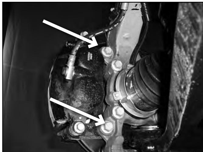
7. Remove the brake rotor and set aside.
