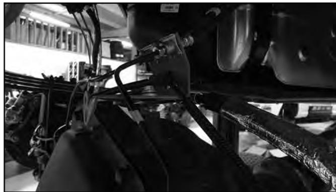
71. Disconnect the ABS line from the frame mount on the driver's side. Retain mounting hardware.
