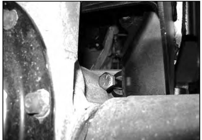
31. Fasten the support bracket to the rear of diff drop bracket. Fasten with the driver's side rear cross member hardware. Attach the hardware at the differential bracket from the front to rear. Leave all hardware loose at this time. (Fig 20A).
