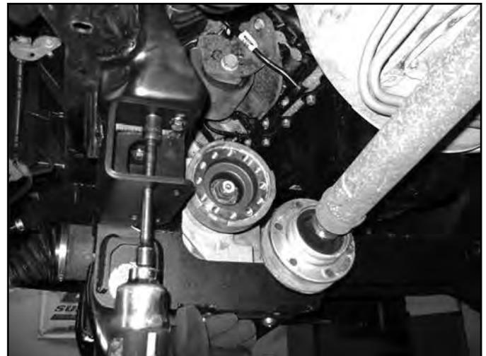
39. With the lower control arms installed torque the four cross member mounting bolts to 222 ft-lbs. Ensure that the front cross member is centered in the vehicle. Torque the differential skid plate bolts to 65 ft-lbs. Tighten sway bar drop hardware to 35 ft-lbs.
