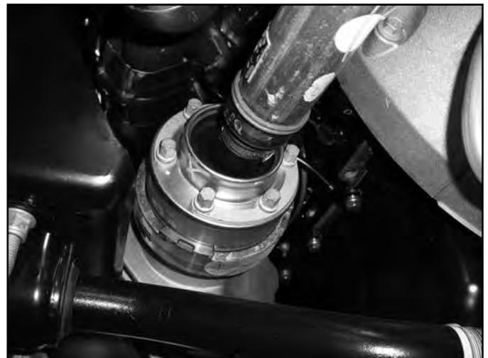
23. Remove the passenger's side CV only. Strike the shaft with a hammer to dislodge it from the splines. This will make handling the differential much easier. (Fig 12)
