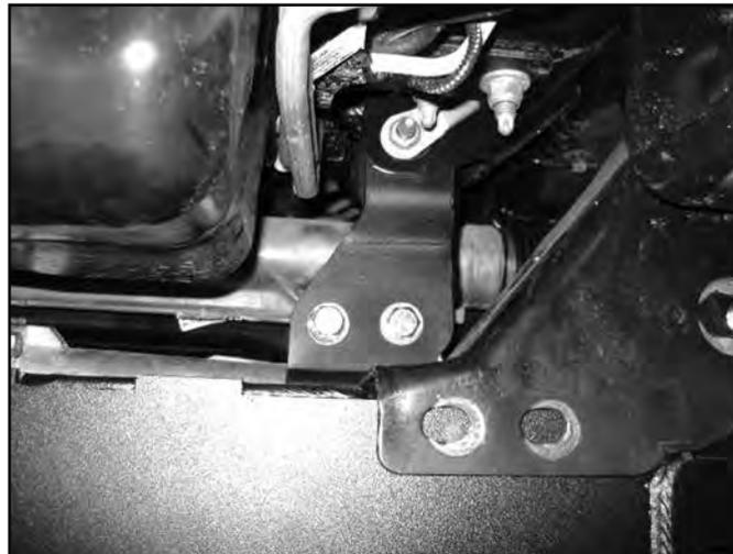
33. Torque all of the differential mounting hardware to 95 ft-lbs (10 total). Attach the differential breather tube. Remove the differential breather elbow from the plastic line and replace it with the provided hose and attach it to the differential.
