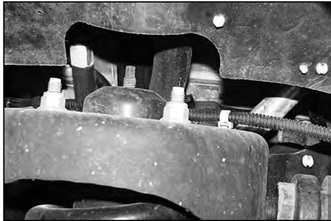
15. Remove the upper and lower ball joint nuts, refrain from hitting the aluminum steering knuckle, use appropriate tool to separate ball joints, avoid damaging the threads.
