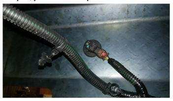
18. On the driver side end cap, there is a knock-out plug. If you have a diesel motor punch out the opening to install the block heater plug.
