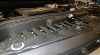
3. Disconnect the sensor/fog light wiring harness. Also, if vehicle is installed with a front camera, unhook the connector. The grille can then be removed by remove (4) 10mm bolts on top and pulling the grille away from the truck to release the clips.
