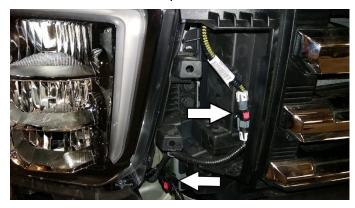
4. Remove the factory bumper side brackets. There will be (3) 15mm bolts on each side.
