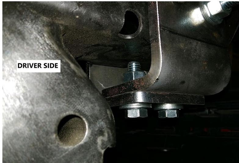
9. Mount the grill guard to the outside of the mounting brackets. Use black carriage bolt and 1/2" hardware to install. Level grill guard and tight all bolts.
