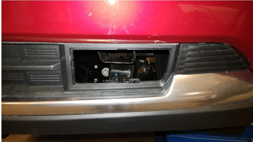
4. Use the Driver Tow Hook Cover for a template to cut the passenger side. Center and mark area to cut.
