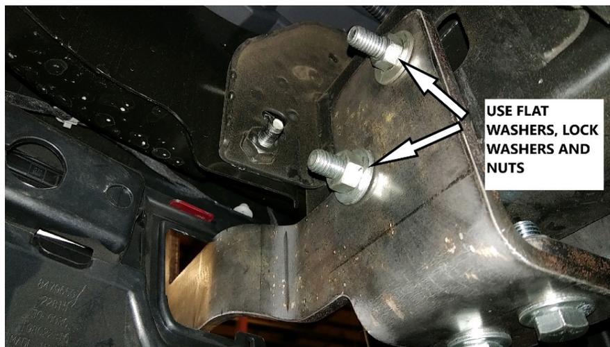
6. Center the brackets through the bumper opening and tighten bolts.
