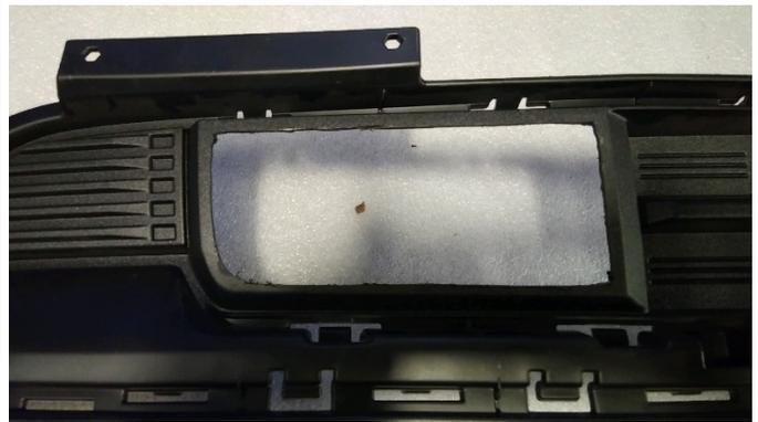
5. There is a driver and passenger side mounting bracket. Mount the brackets to the outer side of the frames. Use 7/16" hardware for the front hole and 3/8" bolt tab and hardware for the back hole. (Photo shown without lock washers)
