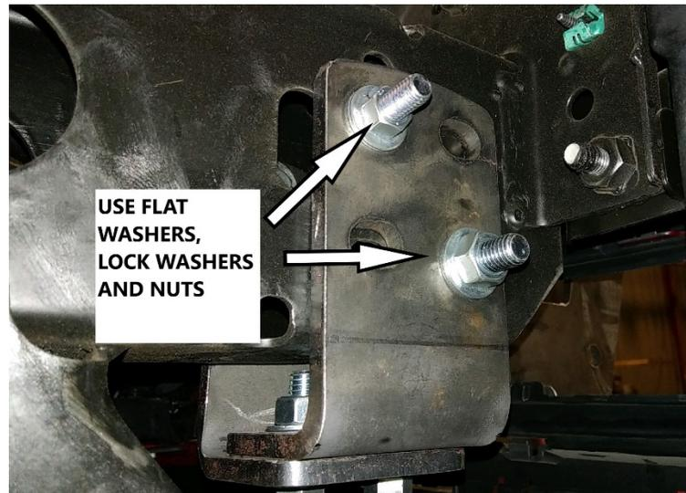
8. Mount the secondary bracket to the mounting bracket using 7/16" hardware.
