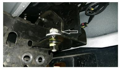
2. (*Diesel*) Remove the bracket that attaches the air dam to the frame. Also, remove the rectangle tubing from the frame.
