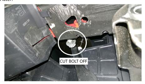
4. Remove the tow hook along with the plastic cover around it.
