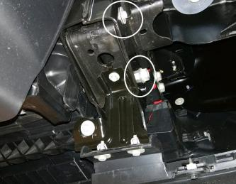
3. (Diesel) On the driver's side, cut the front tow hook's bolt off. You will use a  $\frac{1}{2}$ " x 4" bolt to reinstall the tow hook later.
