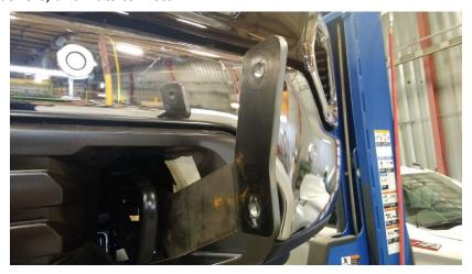
9. Reinstall the tow hooks. Use the factory tow hook bolts. (*Diesel*) Use ½" x 4" bolt. If there are no tow hooks present, use ½" bolts. Also, at this time tighten the 18mm bolt that was loosened in step 1.
