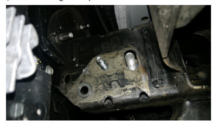
8. From the backside, slide the mounting bracket through the tow hook opening. Use 3/8" and  $\frac{1}{2}$ " washers, lock washers, and nuts to install.
