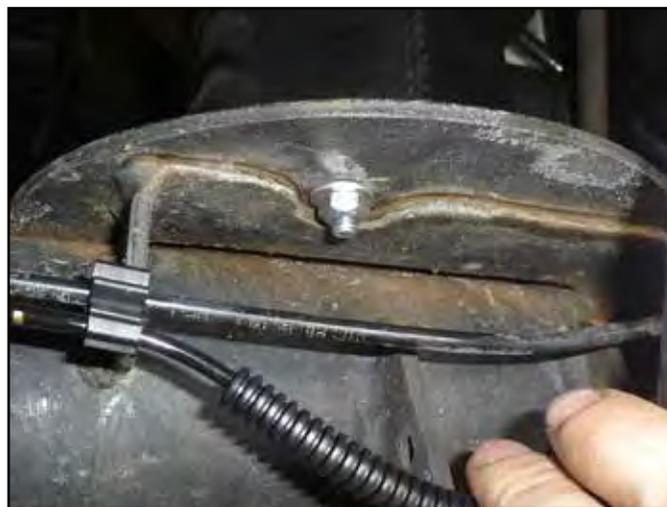
7. Remove the factory shocks, retain all mounting hardware.
