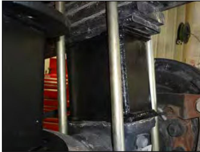
12. Install the provided air bag spacer to the axle with the provided 5/16" hardware from Bolt Pack 606. The air bag spacer will install the same way as the block with the small end of the spacer towards the front of the vehicle (Fig. 8 & 9). The spacers are not side specific and will mount concentric with the axle mount.
