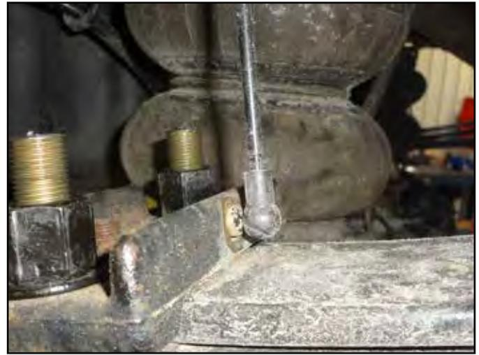
10. **4" Kits ONLY:** Lower the axle and removed the factory plastic center pin. Replace with new metal pin. The pin will be a press fit. It may be necessary to take a rotary grinding tool to remove the sharp edge from the leaf pack to allow easier installation (Fig 6).
