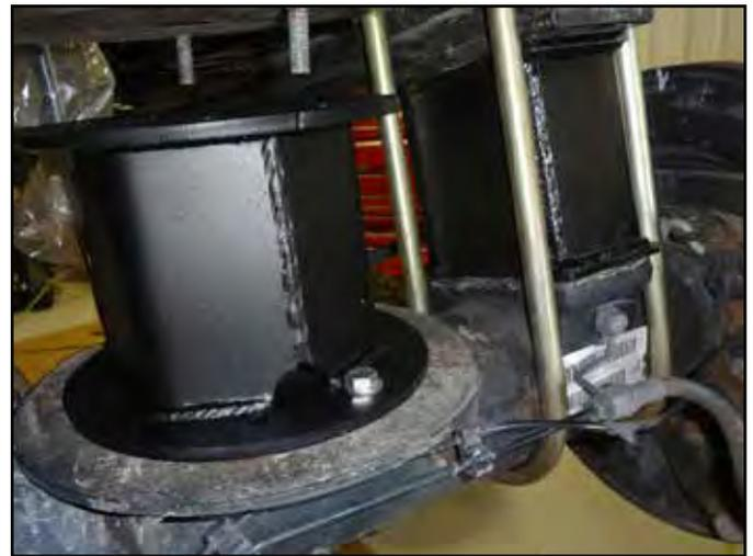
13. Repeat block, spacer, U-bolt, and pin installation on opposite side of the vehicle.
