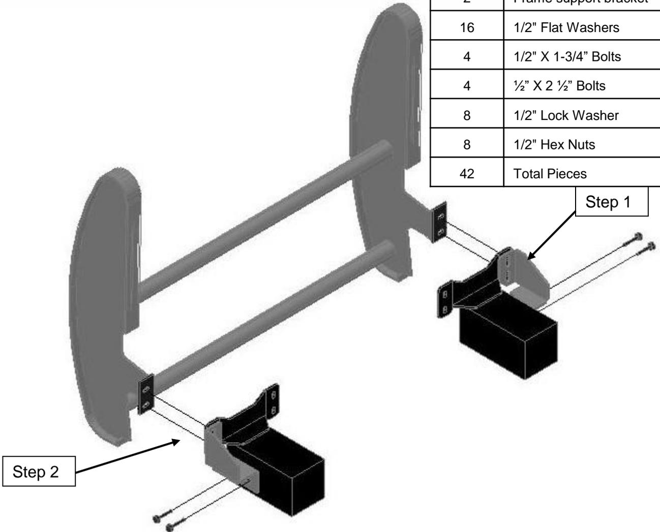
**Step 1:** Install frame support bracket behind frame horn and to lower two bolts on the side of the truck frame as shown. If these two bolts are missing use the two 1/2" X 1 3/4" bolts provided.
