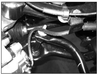
17. Reattach ABS wire to factory mounting clips and brackets. It may be necessary to slide the ABS wire in the rubber grommets to get adequate clearance / routing of the wire. Use silicone spray to allow the grommet to slide on the ABS wire.
