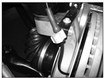
5. Remove the ABS wire from the upper control arm clip. Trim the tab from the factory brake line bracket, do this while the bracket is attached to the arm. (Fig 2)
