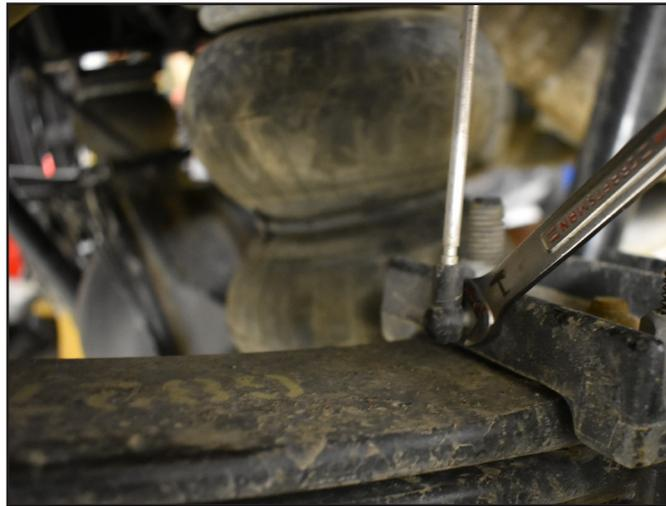
9. Install the provided spacers 136 into the ends of the air bag spacer and place the air bag spacer between the air bag and frame with the U cutout towards the center of the vehicle for the air line. (Fig. 5 & 6). The spacers are not side specific. Fasten with OE hardware and Torque to 89 ft-lbs.
