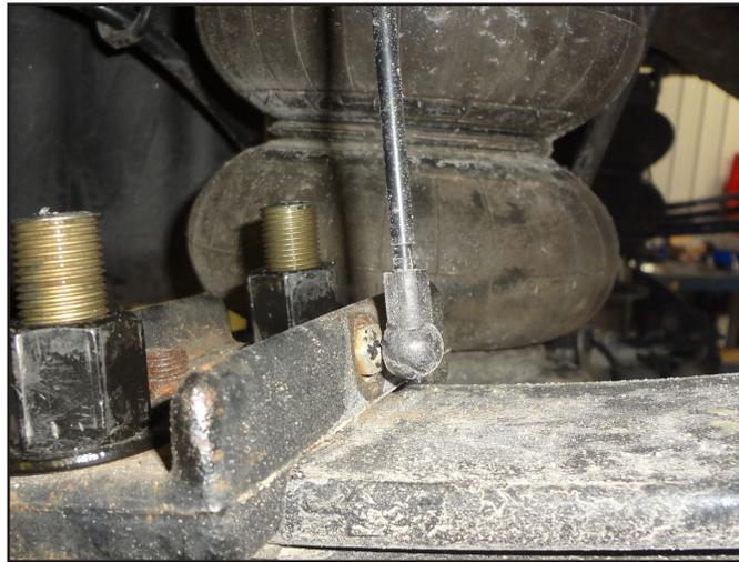
7. Lower the axle and removed the factory plastic center pin be carefull not to over extend the air bag air line. Replace with new metal pin. The pin will be a press fit. It may be necessary to take a rotary grinding tool to remove the sharp edge from the leaf pack to allow easier installation (Fig 3).
