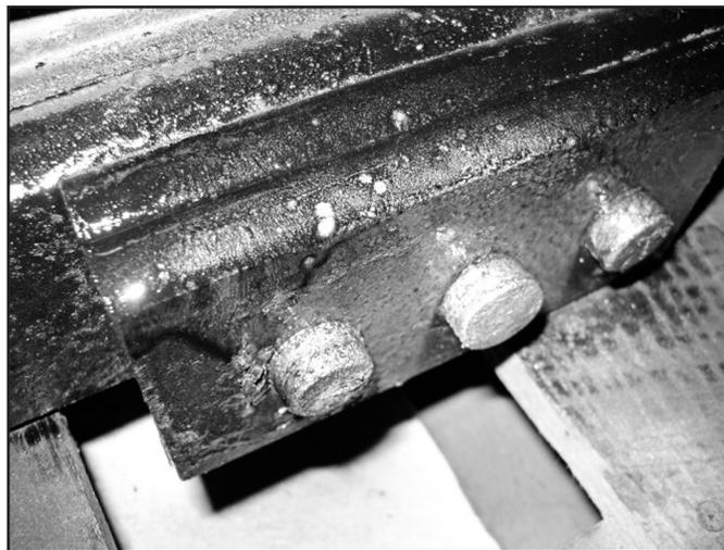
8. Install the new lift block. Install the new U-bolts and install the nuts, but do not tighten at this time.
