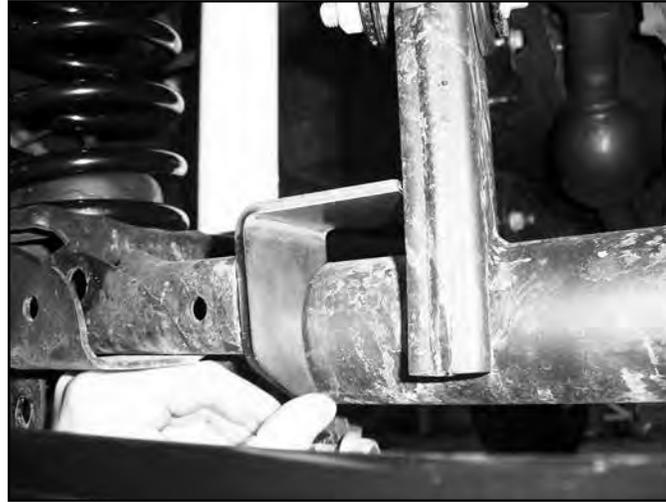
19. Position the new flat track bar mount gusset plate (01942) so that it spans the two passenger's LCA mounting plates and the narrow end butts up against the bottom side of the OE track bar mount. Note the areas to be welded, remove the gusset and remove paint from the areas to be welded (Fig 6). Reposition the gusset and weld in place. Allow all welds to cool and paint the entire area where there is any bare metal.
