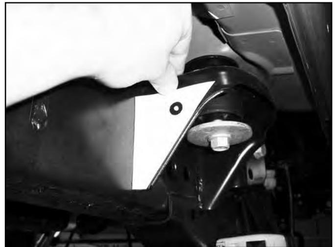
24. Remove the bracket and drill 11/16" holes at each of the 3 marks made on the frame rail. Drill the body mount hole to 1/2". Drill the hole in the bottom of the frame out to 9/16". This will provide clearance for the bolt to pass through with the fish wire attached.
