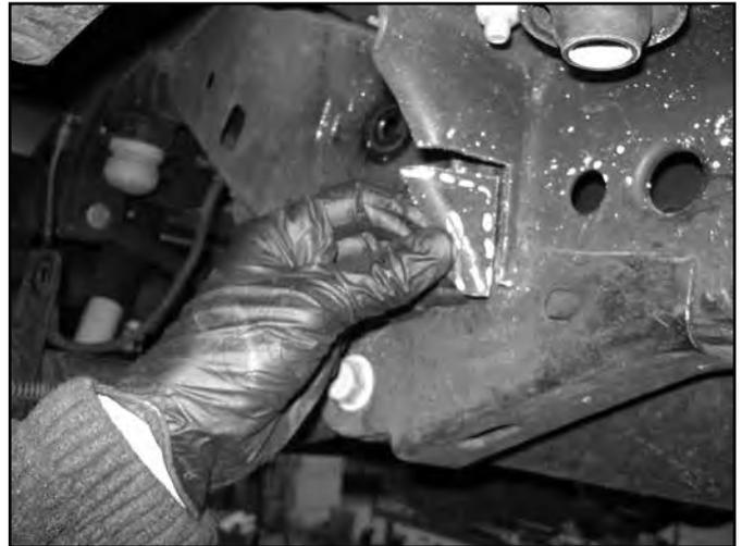
20. Remove the upper control arm pocket from the frame with a sawzall. Trim 1/4"-1/2" away from the frame all of the way up. (Figure 9R, 10R)
