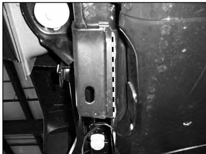
17. After removing the bracket, go back and grind the weld located within the body mount smooth 1" from the end. This will allow the new mounting bracket to lay flush against the frame when installed. (Fig 6R)
