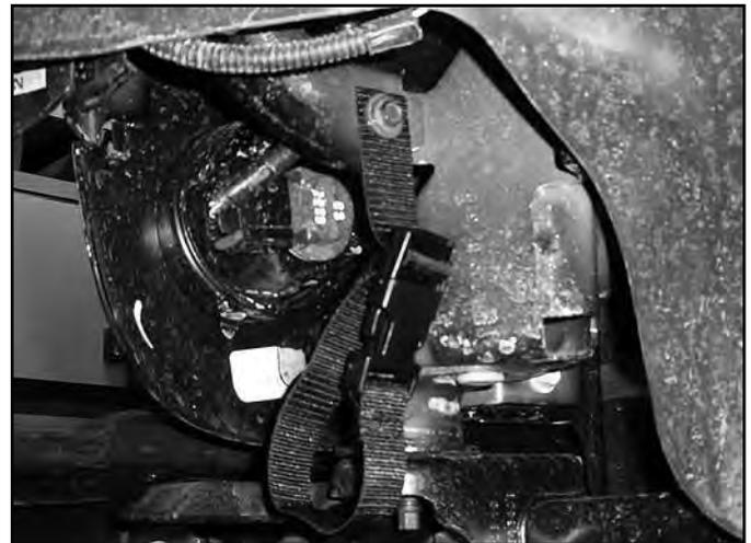
56. Slide the male clip up the lanyard and attach the female clip to it (Fig 23). This will be the stowed position for the lanyard when not it use (when the sway bar is connected)
