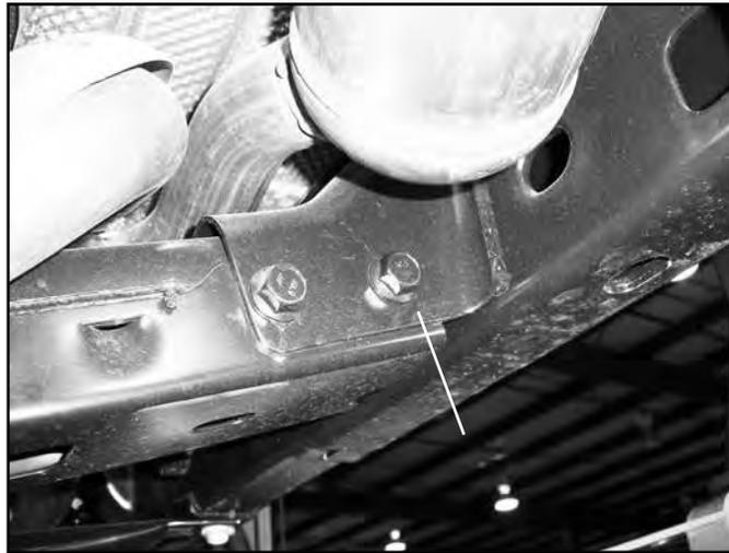
24. Position the provided front LCA mount (01983B-drv, 01984B-pass) up to the frame rail and against the front face of the transmission crossmember (Fig 11). Loosely fasten the bracket to the frame with the OE skid plate bolt and to the crossmember with the OE crossmember hardware.
