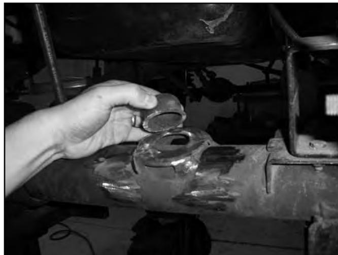
41. Locate the new provided coil mounts. Place the mounts over the factory mounts so that the new mount wraps around the back side of the axle tube and is centered over the factory mount (Fig 22R, 23R). Note the areas to be welded on each side of the mount to the axle and at the front where the new mount rests on the factory one.
