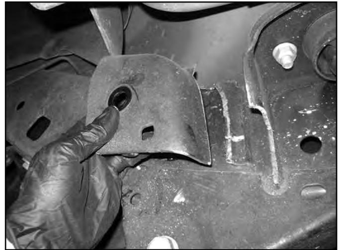
21. Remove gas tank skid plate bolt located just ahead of the factory lower control arm mount. Retain skid plate bolt.
