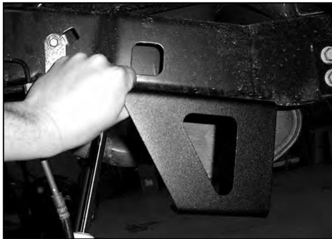
47. Remove bracket and drill a 11/32" hole at the mark.
