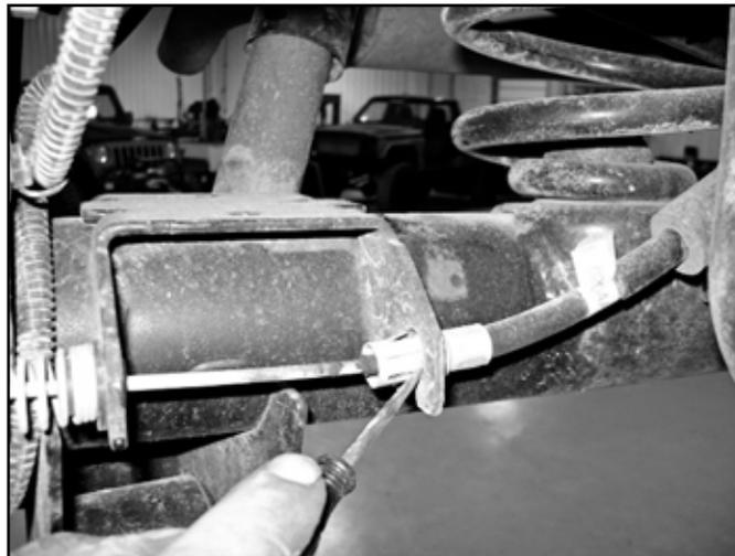
6. Disconnect the rear driveshaft from the axle. Retain hardware. *Note: Depending on the lift amount being installed and the vehicle model, the rear driveshaft may need to be replaced. If this is the case remove the driveshaft from the transfer case as well.*
