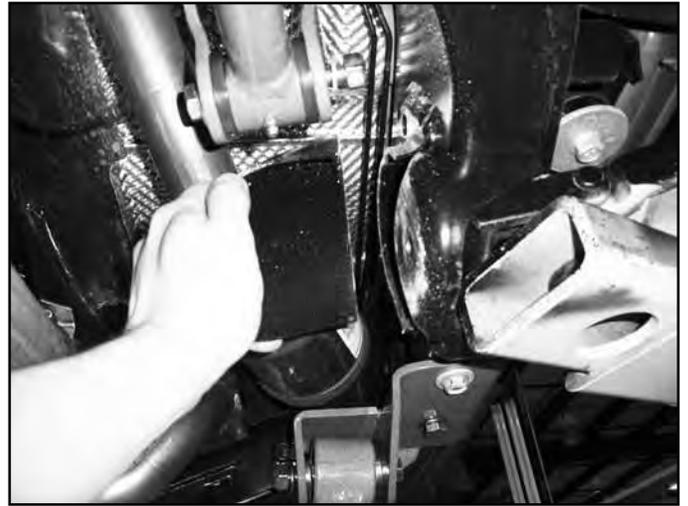
30. Cut the passenger's side factory LCA mount in the same manner as the driver's side.
