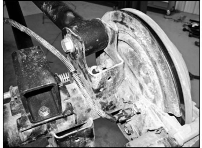
63. Attach new brake lines 'L' bracket to the frame rail with OE hardware. Tighten hardware securely.
