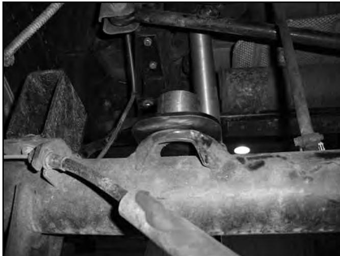
42. Remove the new coil mounts and remove any paint, rust, oil, etc from the areas to be welded.
