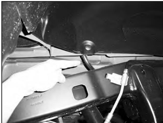
11. Support the axle, disconnect the shocks at the axle. Retain hardware.
