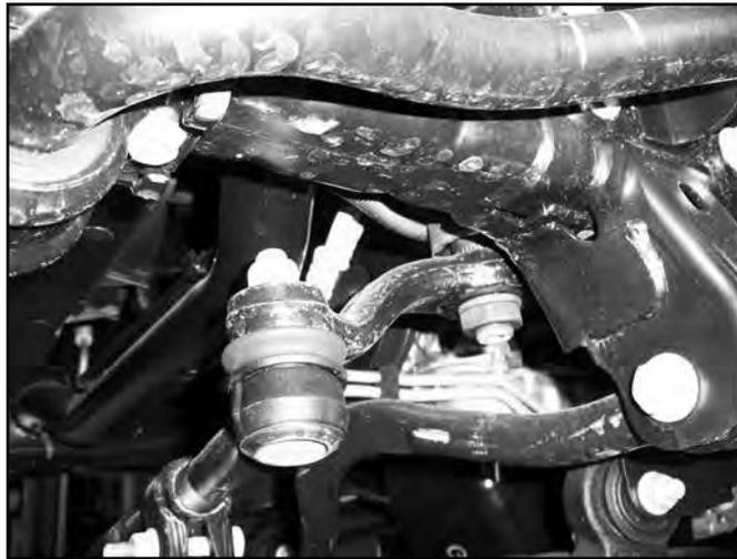
9. Make indexing marks on the pitman arm to indicate the position relative to the splines. Remove pitman arm from steering box with appropriate puller. Retain hardware.
